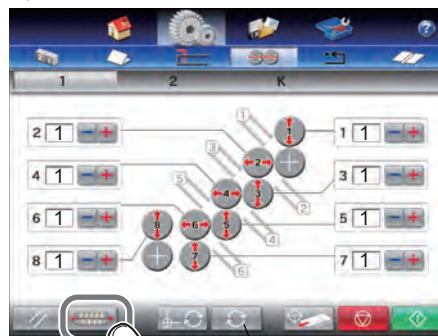
▼ Roller Gap Screen : Example of 6 buckle chutes
