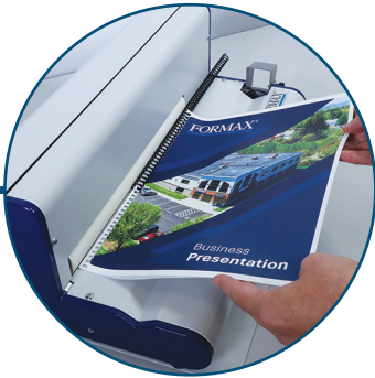
Electric Coil Inserter Convenient rubber roller effortlessly inserts plastic coils.
