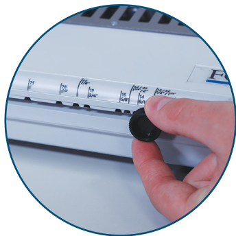
Quick-Adjust Comb Dimensions Change settings in seconds
