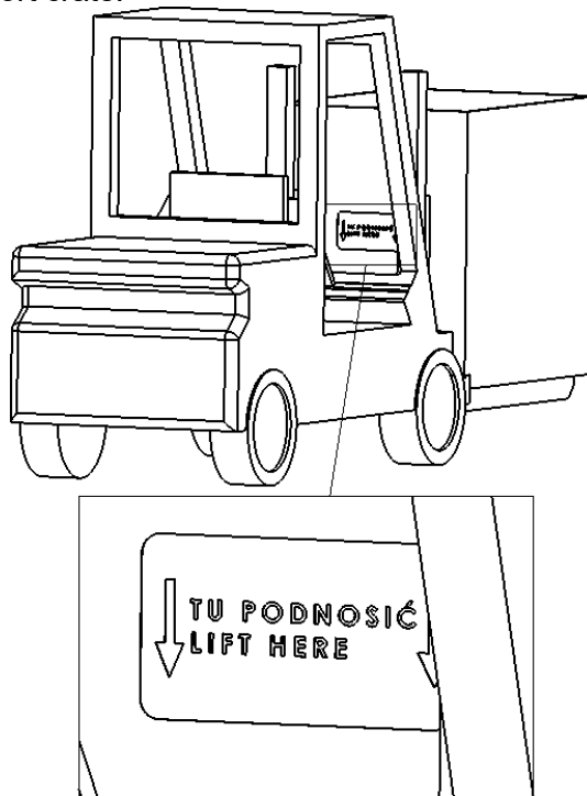
Figure 5a. Transporting the cutter in the crate using a forklift.
