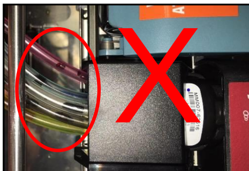
BAD – Do NOT use Printer (Empty Tubes or lots of air in tubes)
