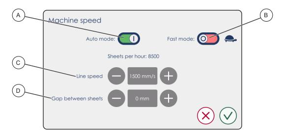
Auto Mode [A] is always turned on by default and it will allow the machine to perform correctly for the majority of jobs.
