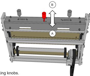
4. Tighten the locking knobs.
