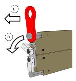
8. Attach Blade Links and Bridge to new blade set and reinsert.
