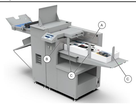
1. Take a stack of printed paper and place it on the feeder table in the desired orientation.
