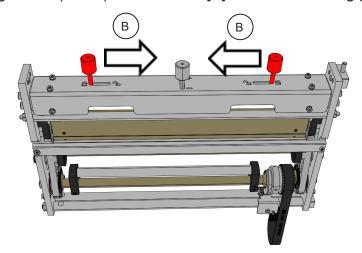
6. Pull the blade set upwards to remove it [C].
