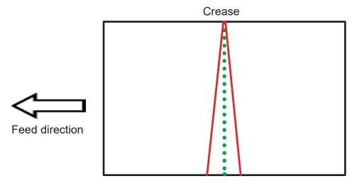
3. To adjust crease skew, loosen the crease adjustment knob by rotating it counterclockwise.
