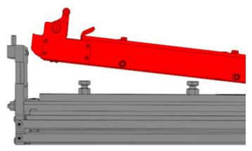
5. Pull the blade set upwards to remove it.
