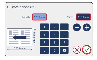
Push on Length and Width to enter the desired custom size. Push the green tick mark to confirm.
