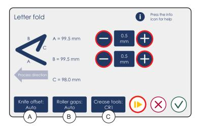
4. Each pattern has an adjustment screen that allows making small corrections to crease positions to achieve the desired output. Use the +/- buttons to make the adjustment and press the Proof button to run another proof sheet. When satisfied tap the green tick mark.
