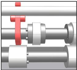
NOTE:Use an 80 gsm sheet of paper to set the 0.1 mm (0.004") gap between the blade and the anvil. Do not force the blade against the anvil to prevent damage.
