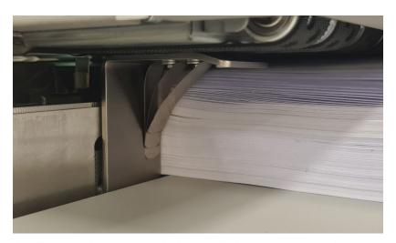
4. Ensure that the guide is parallel to the paper pile.
