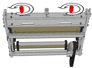
3. Adjust pressure lever on the DynaCrease bridge as shown (A – shallower crease, B – deeper crease).
