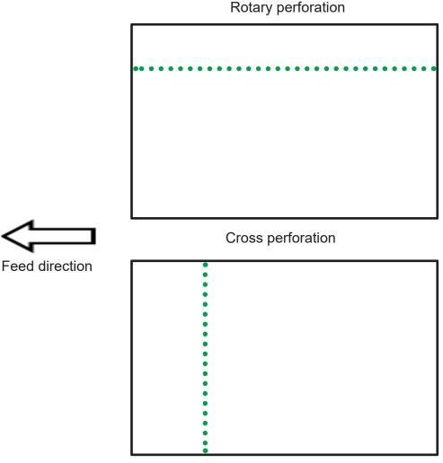
Depending on paper type and the desired finish several different perforation types are available with varying number of teeth per inch (TPI):
