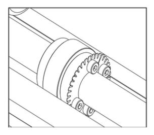
5. Using a 2 mm hex key loosen one of the drive hubs [E] and slide it away from any obstructing drive wheels or hubs in order to mount the anvil.
