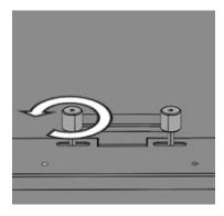
9. Move the knob slightly, either to the left or to the right depending on the direction of the crease skew.
