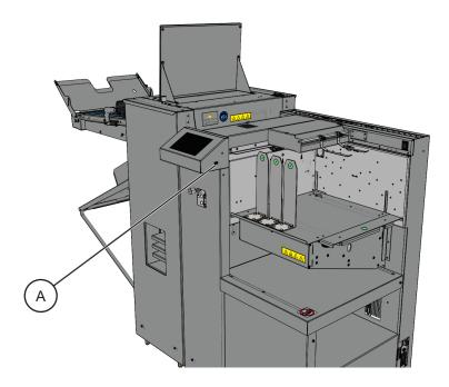
2. With the target machine turned on, insert a USB stick containing the data from the other machine into the USB port [A].
