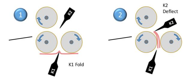
A Half Fold K2 cycle means K1 deflects the paper and K2 folds the paper. This leads to a square spine finish. This cycle is shown below.
