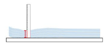
Measure the height of the leading edge of stack of paper: the difference between the leading edge and the lowest point is the amount of paper curl
