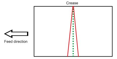
8. To adjust crease skew, loosen the crease adjustment knob by rotating it counterclockwise.
