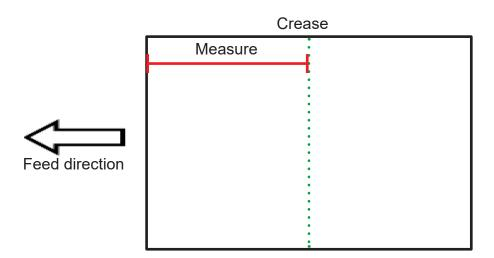
3. If the measurement is not within the machine tolerance ( $\pm$  0.25 mm /  $\pm$  0.01") contact a certified service technician.
