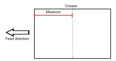
3. If the measurement is not within the machine tolerance ( $\pm$  0.25 mm /  $\pm$  0.001") contact a certified service technician.
