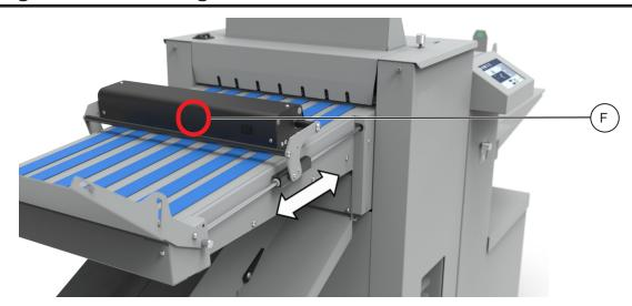
There are two ways to adjust the position of the delivery roller position:
