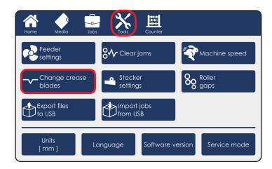
11. Use this menu to choose the blade set that has just been installed and set its direction (crease up or crease down). Tap on the green tick mark to confirm.
