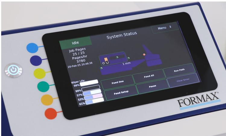
The touchscreen on the printer is a control center for media set-up. It can also be used for monitoring printing as well as pausing and restarting jobs plus recovery for any printing errors. Additionally, it provides the ability to store print jobs and allows the user to view and select print jobs for printing.
