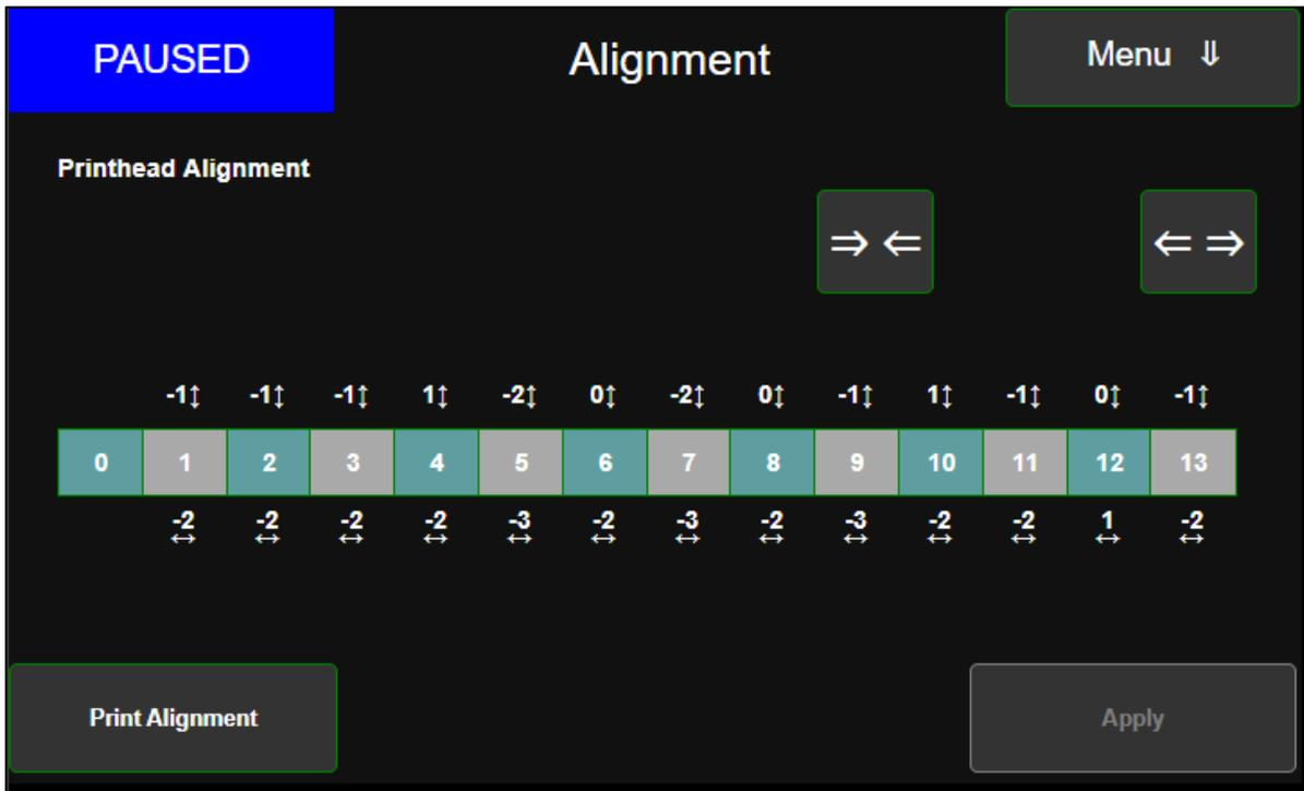
The **Alignment** option is used to view and adjust the settings for printhead alignment.
