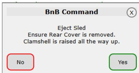
Click on “Yes” to acknowledge that the Sled Access Cover (Rear Cover) is removed, and Clamshell is raised all the way up (12.5mm). The sled will be driven partially out of the print engine, towards the entry end of the printer.
