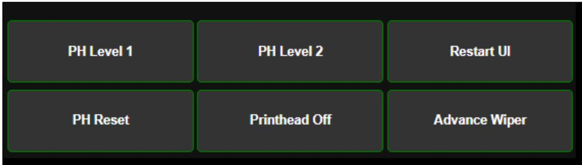
The **Maintenance** page provides selection buttons for maintaining the printhead and wiper.
