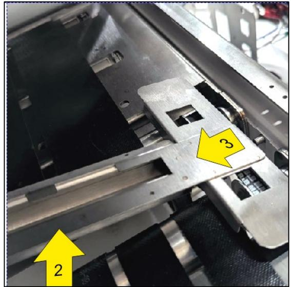
3. Empty the ink and debris from the **Print Platen & Ink Drip Tray Assembly**. Wipe ink from the platen surface. Clean using distilled water and a damp, lint-free cloth.
