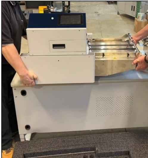
**CAUTION:** Use proper lifting techniques as the Printer weighs ~145 lbs.
