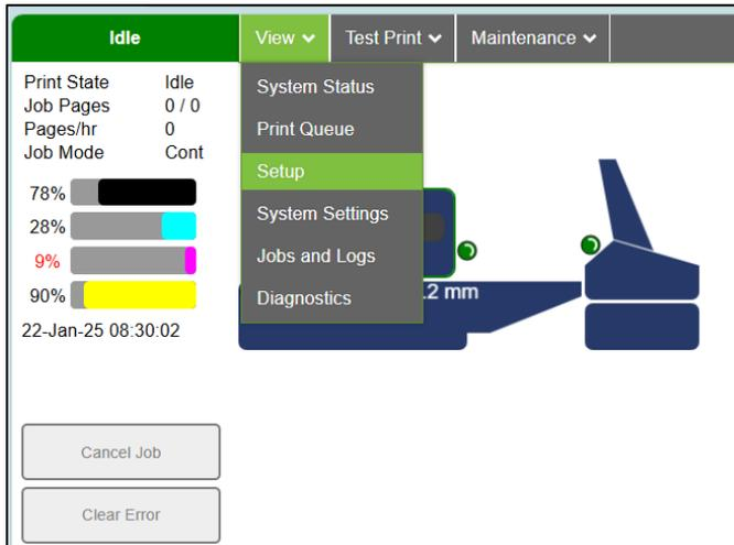
8. From the Setup menu, click on the button labeled “Sled”. Then click on the button labeled “Eject Sled”.
