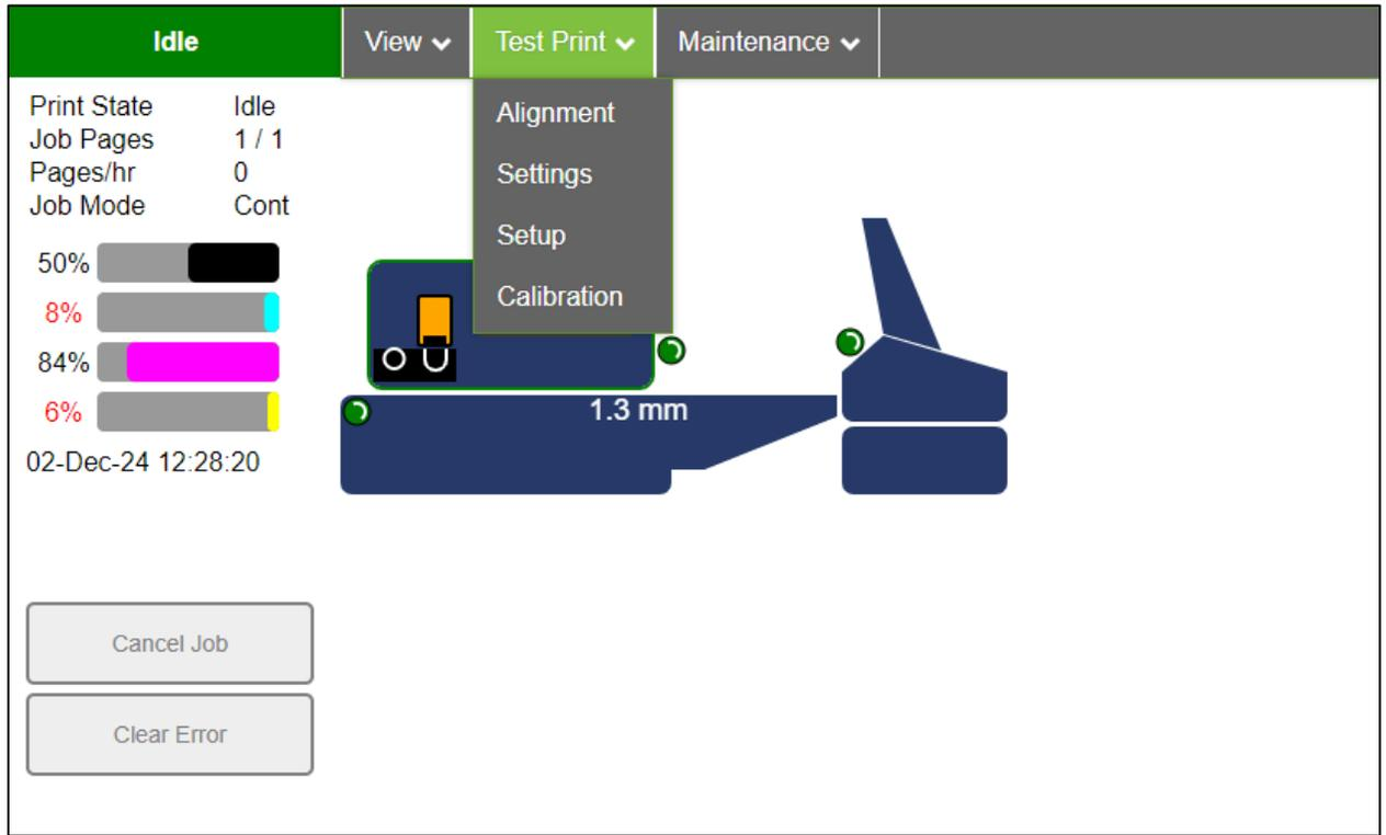
When a test print is selected, a popup box will appear prompting the user to confirm the selected test print is required.
