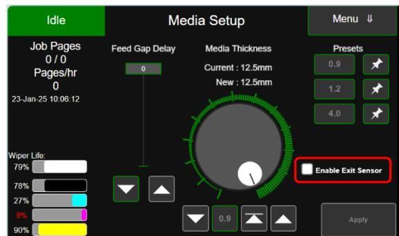
**NOTICE:** By unchecking "Enable Exit Sensor" you are reducing the printer's ability to detect a media feed issue. Therefore, printer transport may continue to run when a paper jam occurs.
