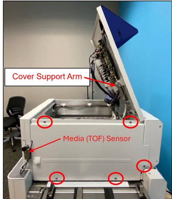
5. Remove the Sled Access Cover, held in place by five Phillips head screws (circled).
