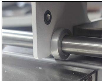
The extensions (stand-offs) at the exit end of the Glide Riser Stand should rest against the printer frame to keep the feeder at the correct distance from the printer and square to the printer frame.
