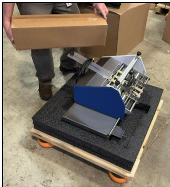
3. Remove the feeder and riser stand from the pallet and place them on a sturdy table. Position feeder and riser stand at right-hand side of table.
