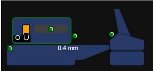
**NOTICE:** A green feeder sensor does not indicate that the feeder is ON. The feeder sensor is driven by the printer, therefore it will function (show green/red), even if the feeder's power is turned OFF.
