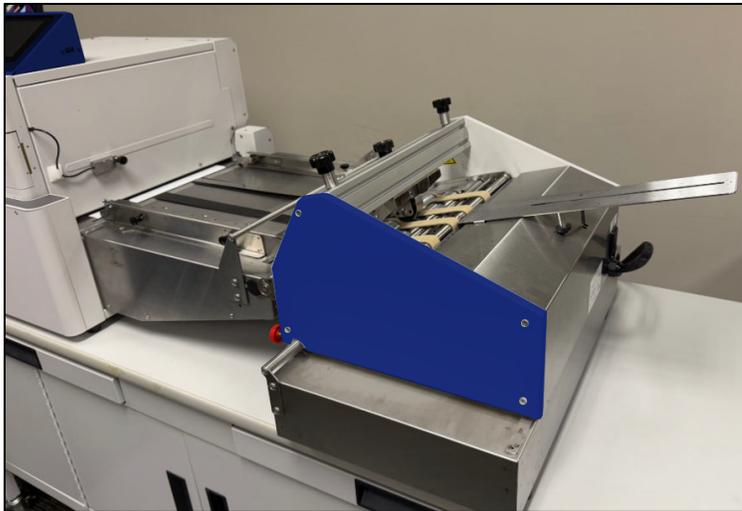
**NOTE:** Make sure exit end of feeder engages with both bushings on Stand shaft. You will need to manually position bushings, so the side of the feeder falls into the corresponding bushing slot at each side of the feeder.
