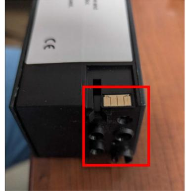
5. Gently place the new cartridge in the empty slot, making sure that the correct side of the cartridge is facing inwards.
