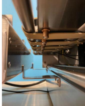
After performing the above alignment, the red knob on the Glide Riser Stand can then be loosened and the feeder position adjusted (feeder can be slid on the Glide Riser Stand) to accommodate the range of media widths that this feeder supports. From 3" to 15" wide media.
