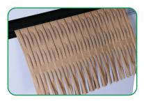
Perforation Transformation Cardboard up to .4" thick is quickly transformed into valuable net-like cushioning packing material
