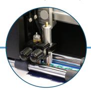
Digital Cutting/Creasing Head Dual-action head applies up to 750gf individually for both cutting and creasing tools
