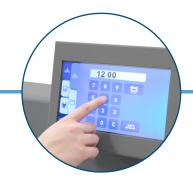
Touchscreen Control Panel Set cutting lengths, program and save up to 99 jobs, up to 30 cuts each
