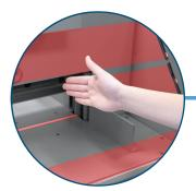
Infrared LED Safety Curtain Immediately stops operation if the light beam is broken
