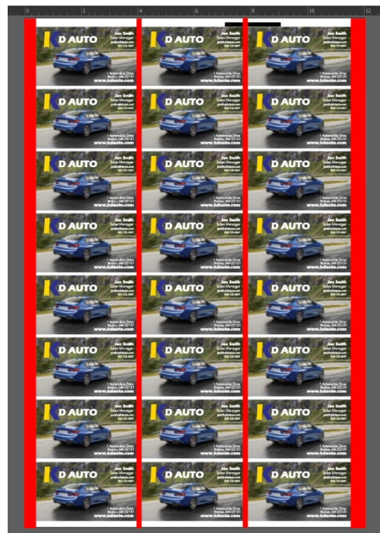
The red highlighted areas are fixed based on the cutting cassette. (width cuts)
