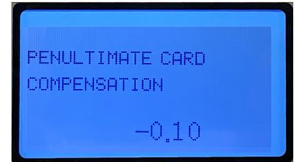
**Third From Last Card Compensation:** Adjusts the cut length of the third to last card individually
