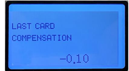
**Penultimate Card Compensation:** Adjusts the cut length of the second to last card individually
