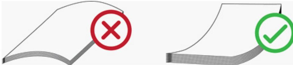
Do not use paper that is curled in this direction (X), known as “laterally curled stock.” This can result in misfeeding, inaccurate cutting and paper jams.
