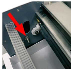
4. Align blade cassette notch with mounting pin
