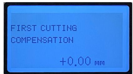
**Mark Position Compensation:** Adjusts where the cut is made after the mark
