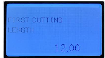
**Mark Position Length:** This setting determines where the first cut will be made from the top edge of the mark. If "Mark" is selected on the job screen it will override the "First Cutting Length" value.
