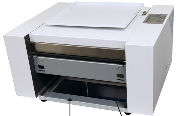
2. Be sure that the waste hole of the cutter aligns with the cabinet waste hole on top of the cabinet to ensure the scraps are caught properly.
