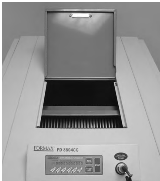
Control Panel and Cutting Block Access Door
