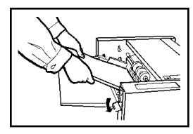
Adjust the paper feed pressure adjustment lever to the thickness of the paper. Usually it is set to "NORMAL."
