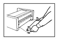
2. Remove the thumb screws (in the circles) and attach the columns on the right and left hooks, then fasten the thumb screws.
