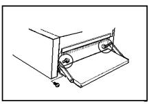
3. Remove the screw (see circled area, right) and install the paper holding plate attachment. Set the paper stopper and paper guides as shown in the picture.
