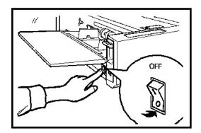
Open the safety cover. Spray the sensor with canned air, or gently clean with a cotton swab to remove paper dust residue.
