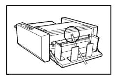
Insert the edge of the support tray into the right and left columns of the paper infeed tray. Then set the support tray downward.
