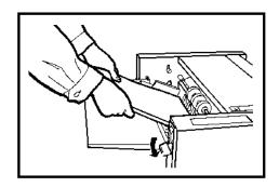
3. Pull out the paper with a hand while feeding it by holding down the JOG key.
