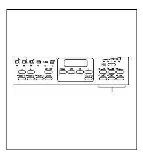
Press and hold the Clear/Reset key, release immediately when the alarm rings once.
