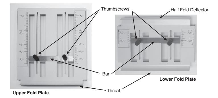
To adjust fold plates to desired fold and length of paper, first loosen the two thumbscrews on each of the two fold plates. Second, align the center bar so the marks on each side of the fold plates match up.
