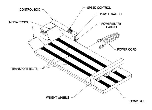
Figure 1.1 – FD 260-20 with Components
