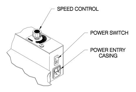
Figure 5.1 -- Adjusting Speed
