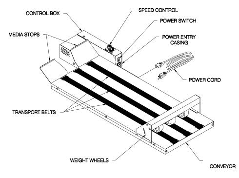
Figure 4.2 -- FD 260-20 with Weight Wheels
