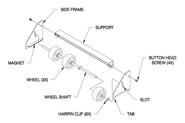
Figure 4.1 -- Assembling the Weight Wheels
