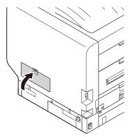
$\mathbf{Q}$  Tighten the access cover screws.
