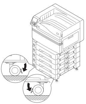
Loosen the nuts (x2) at the top of the feet on the right of the device.
