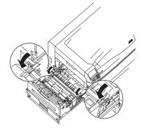
Put the exit unit back into the printer.
