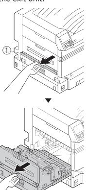
Raise the lock levers (blue) at both ends of the transfer roller unit installation location of the exit unit.
