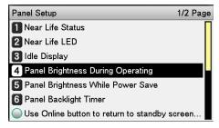
When adjusting the brightness for when in power save, select [Panel Brightness While Power Save], and press the [OK] button.
