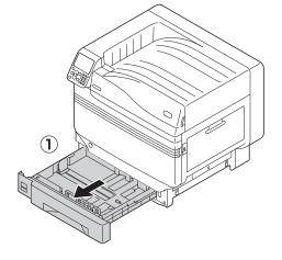
2 Slide the paper guide (1) and paper stopper (2) to align to the size of the paper that has been set.
