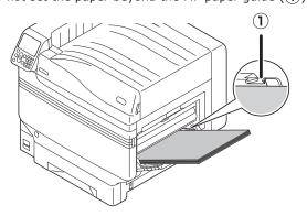
Adjust the paper guide to fit the width of the paper that has been set.
