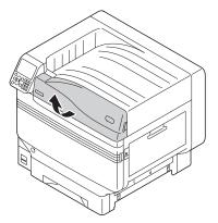
Check the position of the slot that has a label stuck on it with the same letters and colors, and firmly push the toner cartridge in as far as it will go.
