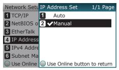
If acquiring the IP address automatically, check that [Auto] has been selected, and then press the [OK] button.
