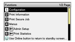
Press the scroll button ▼ several times to select the [Admin Setup], and then press the [OK] button.
