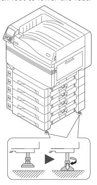
When each foot has reached the ground, tighten the nuts at the top to secure the tray unit.
