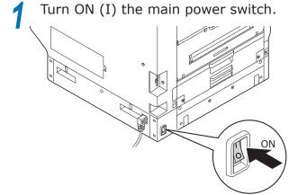
Press and hold the power switch for approx. 1s.
