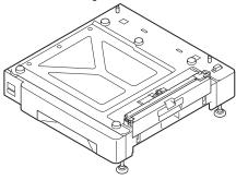
☐ Mounting the expansion tray unit with casters to the main printer unit
