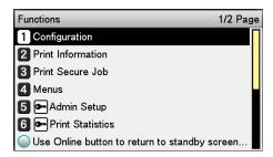
Press the scroll button ▼ several times to select the [Admin Setup], and then press the [OK] button.
