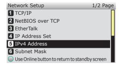
Use either the scroll buttons ▲▼ or the 10-key pad to enter the first 3 digits of the IP address, and then press the [OK] button. Enter the next 3 digits in the same way. When all entries are complete, press the [BACK] button.
