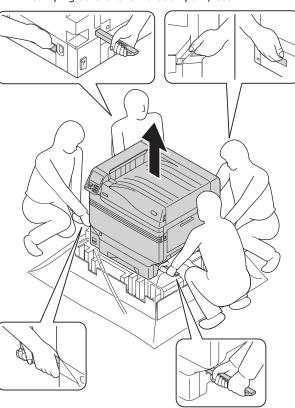
Gently lower the device into its installation location.
