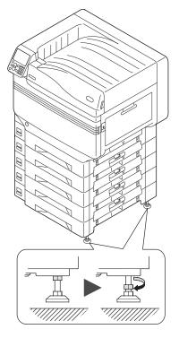
Rotate the nuts and bolts at the bottom of each foot to lower the feet.
