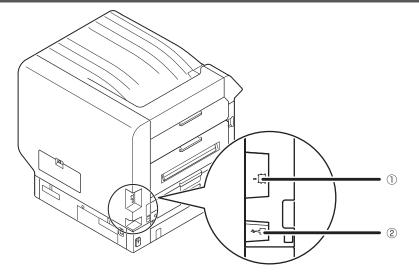
①**LAN (network) Interface Connector** Connects the LAN cable.
