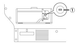
Align the screws (x2) on the built-in HDD to the holes on the device.
