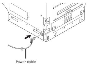
Insert the power plug into the power outlet.
