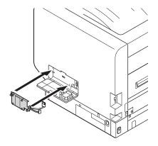
Rotate the screws (x2) in the direction of the arrows to tighten securely.
