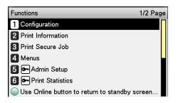
Press the scroll button ▼ several times to select [Admin Setup], and then press the [OK] button.
