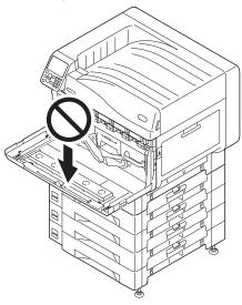
• Do not press on the cassette from above when the cassette is pulled out.
