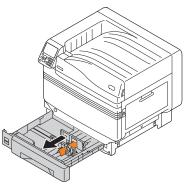
Slide the paper guide and take out the sheet retainer.
