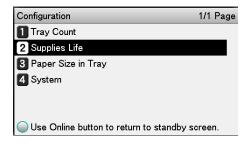
Select the consumable or maintenance unit (image drum, belt unit, fixer unit, or waste toner box) to be checked.
