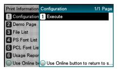
15 Check that the HDD has been added to the "Configuration".
