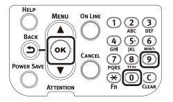
Press the scroll buttons ▲▼ to select the size of the paper that has been set, and press the [OK] button.
