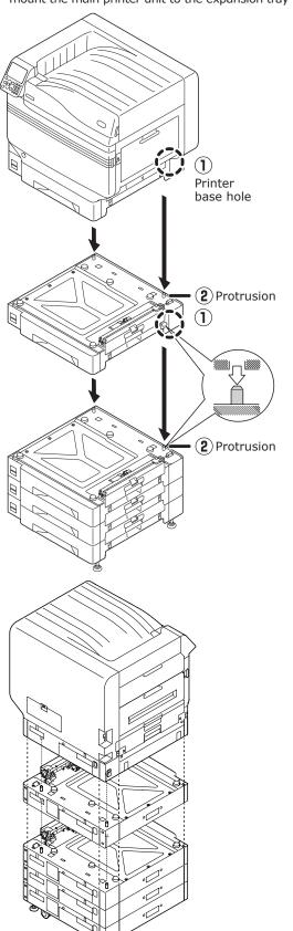
• For the expansion tray unit and large-capacity expansion tray unit with casters, adjust the caster locks (x2) and feet (x2).
