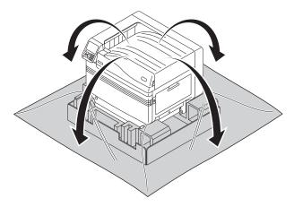
Remove the three carrying levers at the bottom of the printer (1), and check the three locations of the carrying handles (2).
