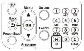
The function number input screen will be displayed, so use the 10-key pad to enter the (3-digit) menu number to be displayed, and then press the [OK] button.
