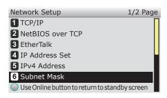
11 Enter the subnet mask in the same way as the IP address. When all entries are complete, press the [BACK] button.
