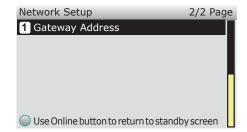
13 Enter the gateway address in the same way as the IP address. When all entries are complete, press the [BACK] button.
