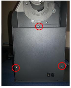
3. Once the screws have been removed, remove the plate
