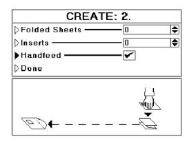
To run daily post, load feed hoppers as required if you have selected additional folded sheets or inserts ('Loading Paper Hoppers' on page 33). Select the job from 'Run Job' on the Main Menu and press the Run button. Insert the daily post documents into the handfeed tray on the folder as shown below - the forms will then automatically be fed and the machine will await further documents. Note that the tower folder is shown – feeder folder is similar principle, but design is different.
