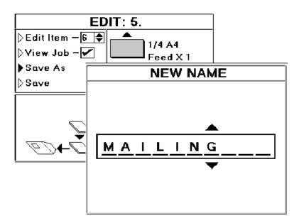
Use the Scroll Up/Down buttons to select the first character, then press  $\checkmark$ . This moves to the second character, and so on, up to the maximum 10 characters. When finished, press x to exit the screen. Confirm your changes, and your new job is now saved and will appear on the Run Job menu.
