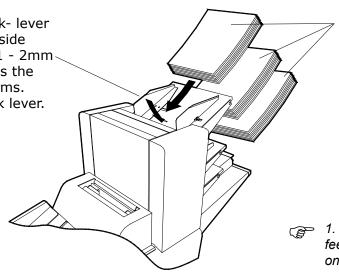
Press down on the tray and load the fanned stack of forms. Ensure that the leading edges are firmly contacting the chassis bridge at the lower end of the tray. Use the indicator lights on the rear edge to orientate the paper.
