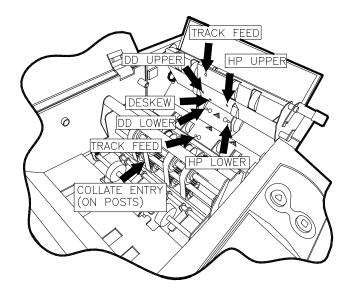
Lower the feeder side cover and raise the top cover. Swing the green latch upwards to raise the roller platten.
