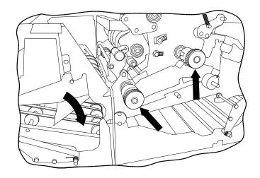
3. Turn the green knobs on the tower feeder to wind the crashed document into the cavity ahead – it can then be easily removed.
