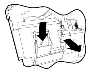
Withdraw the tank by using the green tab
