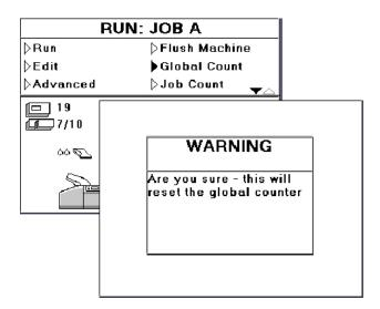
If you are sure you want to zero the count, press  $\checkmark$ . This will reset the appropriate count shown above. Note that the machine's internal count is **not** reset. This count can be seen in Supervisor mode (see page 30).
