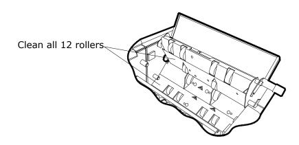
To access tower folder rollers, open the LH side covers and use the green latches to open the daily-post hopper and paper path platten. Also open the front cover using the black latch on the top edge.
