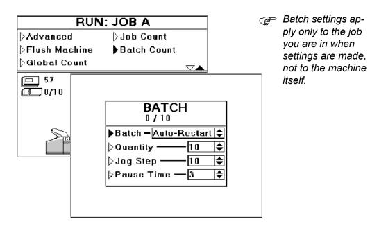
For 'Batch', select 'Auto-restart' (machine will pause for a set length of time and then restart - see below for 'Pause time') or 'Pause' (machine will stop and will only restart when the Run button is pressed).
