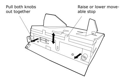
4. Ensure both knobs are properly located before replacing the tray.
