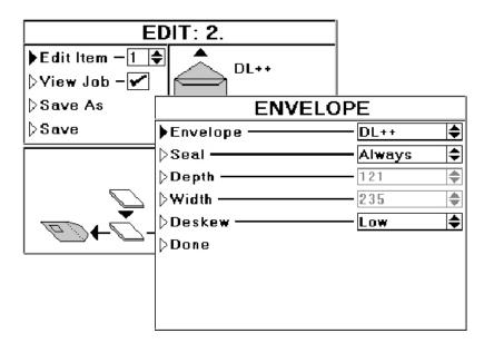
Select the envelope from the standard range, or 'Custom' (this allows depth and width to be set). Choose whether flap is to be sealed always, by OMR select, no seal with flap closed or no seal with flap open. Select required deskew level (high slows machine more). Select 'Done when finished to return to the Edit screen. **Note:** If you wish these settings to be default, see 'Supervisor Mode' on page 30.
