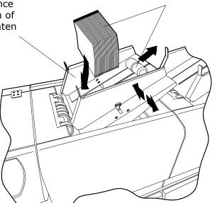
Pull the weighted roller back and load the inserts, ensuring they are fully down. Release the weighted roller so that it 'tips' the inserts into the pickup roller. An alternative heavier roller is also available (part no. C3656A) which can improve feeding of thick booklets. This must be fitted by an Authorised Service Engineer.
