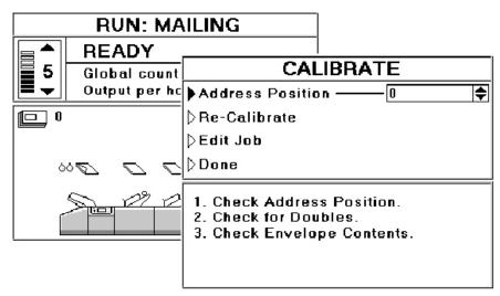
As the calibration is performed on each loaded hopper, check the filled envelope to confirm that only one document per hopper has been fed. If in doubt, select 'Recalibrate'. Also check the address position in the envelope - if it is too far up or down, this can be adjusted to suit. Positive numbers move the address upwards. If you adjust the position, select 'Recalibrate' to check it is now correct.
