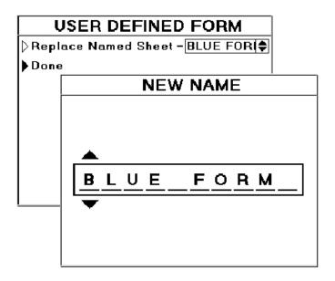
Select the named sheet you wish to replace, then 'Done'. When the New Name screen appears, use the Scroll Up/Down buttons to select the first character, then press  $\checkmark$ . This moves to the second character, and so on, up to the maximum 10 characters. When finished, press x to exit the screen. Confirm your changes, and your new template is now saved.
