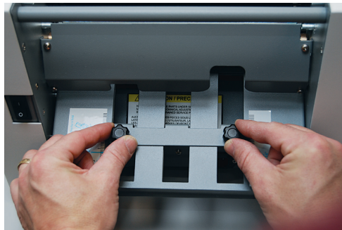
Fig. 2b Adjusting lower fold plate
