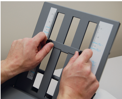
Fig. 2a Adjusting upper fold plate
