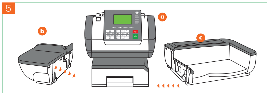
5 Lift the mailing system base (a) slightly on the left hand side and align the hooks to attach the feeding table (b). Attach the catch tray (c) to the right hand side of the mailing system base (a).
