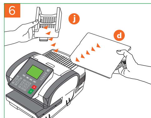
6 Attach shelf (j) to the top of the mailing system base (a). Then attach weighing platform (d).
