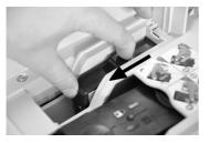
6. Remove the meter from the Mailing System base.
