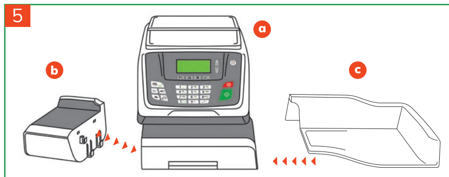
Lift the mailing system base (a) slightly on the left hand side and align the hooks to attach the feeding table (b). Attach the catch tray (c) to the right hand side of the mailing system base.
