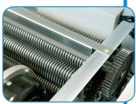
Solid steel gears, heat-treated cutting blades, AC geared motor
