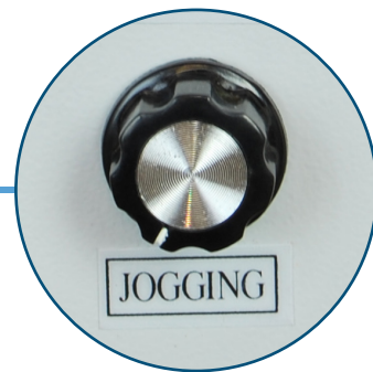
Variable Jog Speed Up to 2,500 vibrations per minute, adjustable for heavy stock
