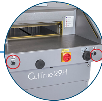
Two-Hand Operation Automatically engages clamp and blade keeping hands away from the cutting blade
