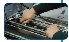
The quick release mechanism allows users to change blades in under 30 seconds, without the need for tools
