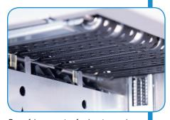
Powerful vacuum top-feed system and optical sensors control sheet separation and make adjustments on-the-fly
