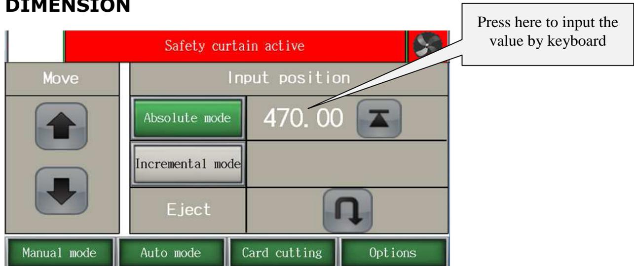
To input the required dimension press the dimension on screen and input value by keyboard. Confirm by pressing **ENT** button and press
