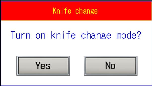
Confirm and make a cut to put the knife into the lower position. After knife change (please look into operator manual for procedure) press the **Knife change** button again,
