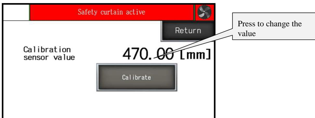
*When starting machine the operator should measure the paper cut and compare with the actual display indication. If both dimensions do not correspond to each other input the base correction.*
