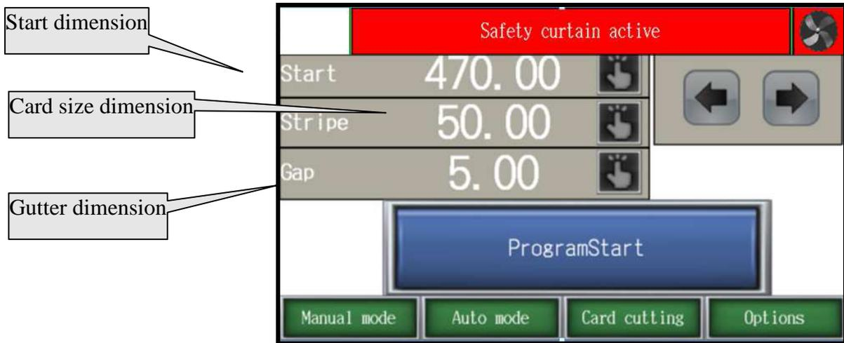
**Start dimension** -first cut dimension starting the card cutting sequence
