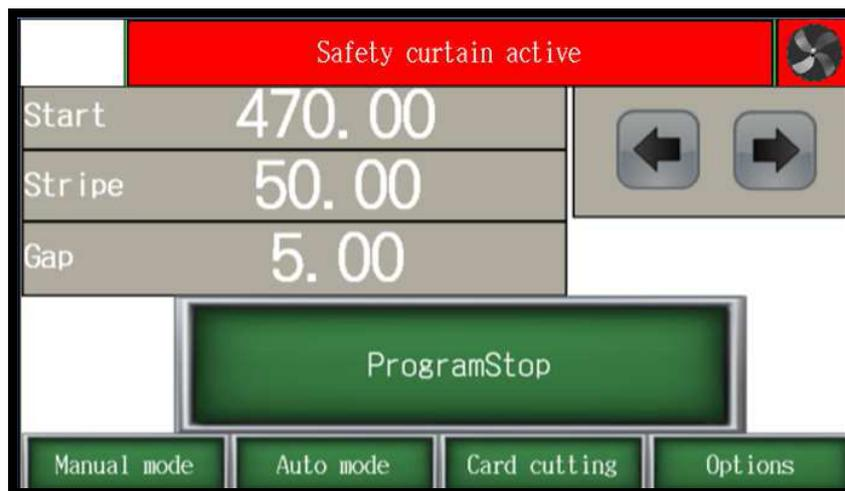
The backgauge moves to the starting dimension and a cut is made automatically.
