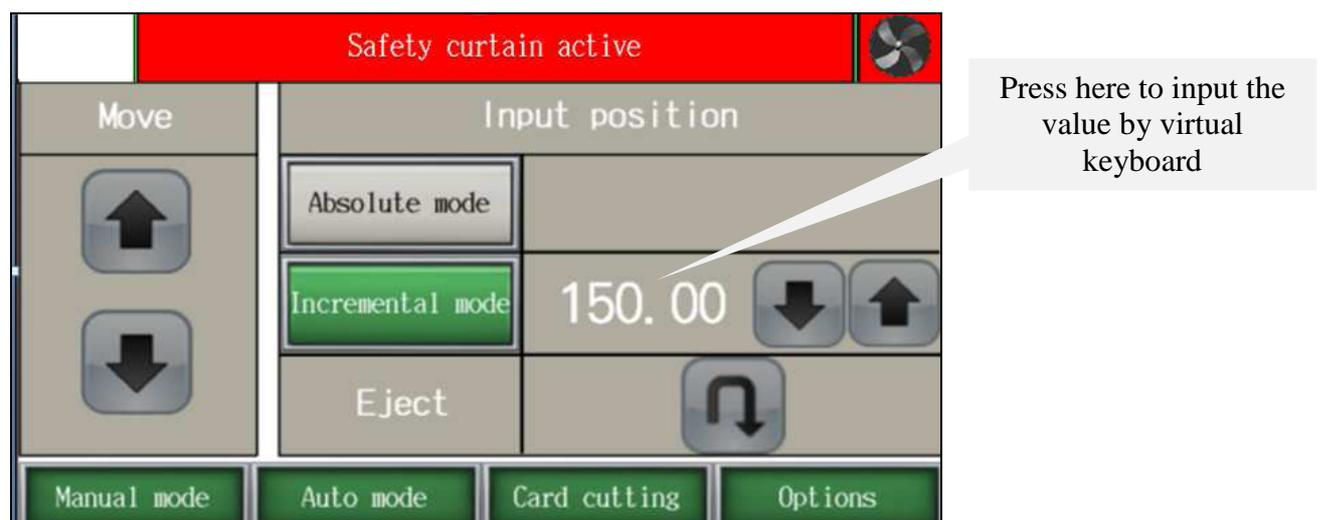
To move the backgauge multiple times by the same dimension (forwards or backwards) input this dimension by pressing it on the screen.
