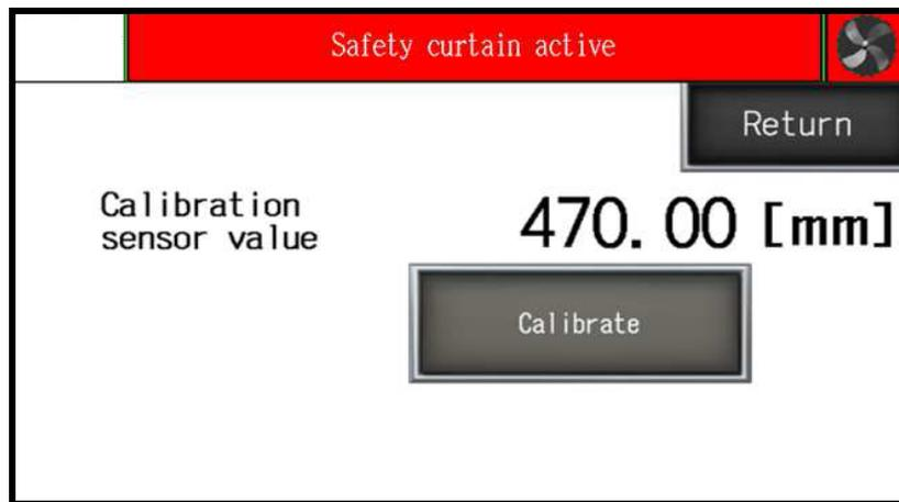
**Calibration**– allows to repeat calibration without machine turn off and dimension correction if needed. (see **5.3 Base correction**)
