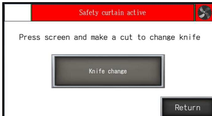
*After pressing, text on screen appears to confirm **Turn on knife change mode?***
