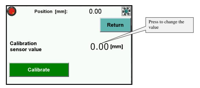
When starting machine operator should measure the paper cut and compare with actual display indication. If both dimensions do not correspond to each other input the base correction.
