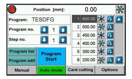
After each cut, the backgauge moves to the next step. When the last cut is made in the selected program the backgauge automatically moves to step 1 and the program can be repeated.
