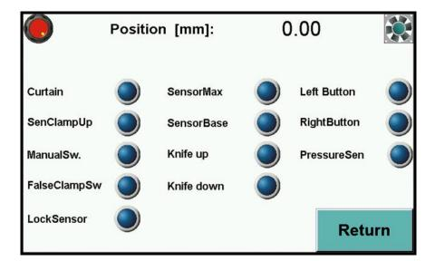
Allows operator to check control system elements like optical sensors, limit switches, buttons, micro swiches.
