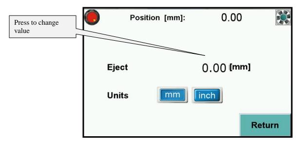
Eject can be set in mm or inches. It is the value by which the paper ream moves forward. After cycle, the backgauge returns to the previous position.
