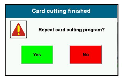
Pressing **YES** moves backgauge automatically into first dimension.
