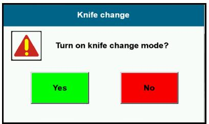
Confirm and make a cut to put knife into lower position.
