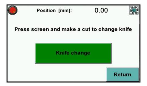
After pressing text on screen appears to confirm **Turn on knife change mode?**
