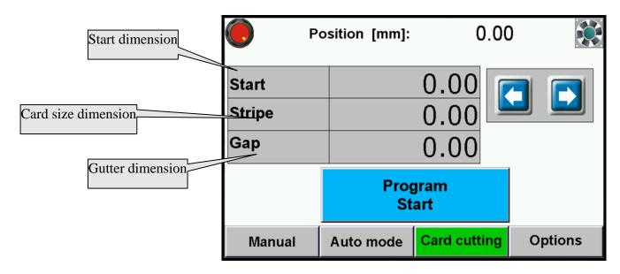
**Start dimension** - first cut dimension starting the card cutting sequence Card dimension – dimension of strip
