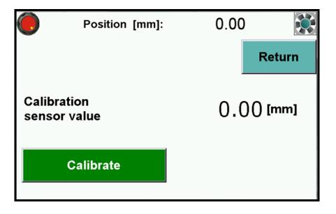
**Calibration** – allows to repeat calibration without machine turn off and dimension correction if needed. (see 5.3 Base correction)
