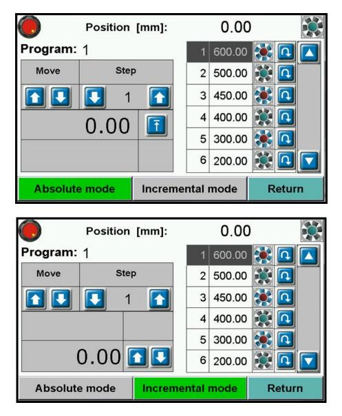
To exit the program edit mode by making a cut, press the Return button to return to the main menu.
