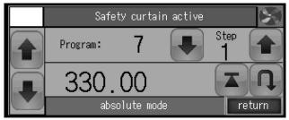
The dimension where the cut was made is saved automatically as a step dimension in the current program. After each cut, program automatically moves to the next step.
