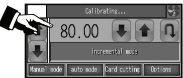
To move the back gauge in increments by the same dimension multiple times (forward or back), input this dimension by pressing it on the screen and using the on-screen keyboard.
