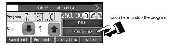
After each cut, the back gauge moves to the next step. When the last cut is made in the selected program, the back gauge automatically returns to Step 1 and the program can be repeated.
