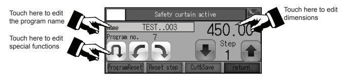
To enter a new program name or change the existing name, press the Name window. The on-screen keyboard will open.
