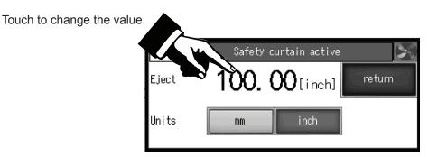
Eject can be set in inches or mm. It is the value by which the paper stack moves forward at the end of a cycle. After each cycle, the back gauge returns to the previous position. Enter the value, then press **RETURN**.
