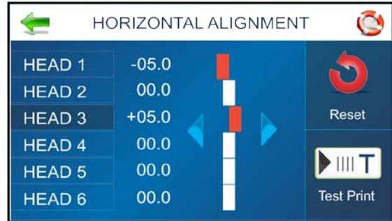
**Heads (1-6):** Align individual Printheads (*side-to-side*) up to  $\pm 100.0$  microns in 5.0 micron increments.
