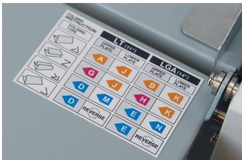
Fold stop position decal on infeed table.
